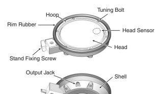
\* Do NOT place your fingers inside the shell, as you may hurt yourself or cause damage to the PDX-8. Or when changing the head, do NOT touch any of the internal parts. Also, do not insert your fingers into the hole of the mounting bracket.
